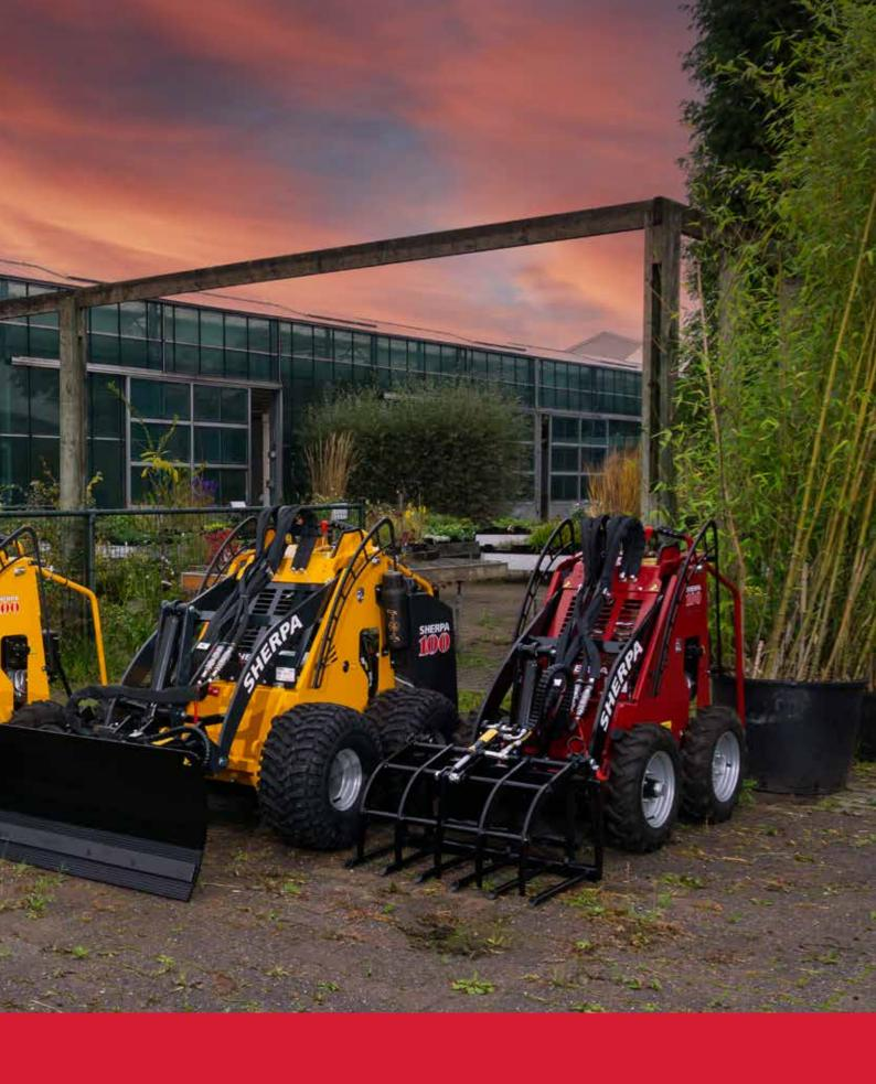
This machine, therefore, is a prime example of working smart! The SHERPA 100 is produced with a width of 76 or 114 centimetres. In 2012, we introduced the first electric skidsteer loader, but the SHERPA 100 is also available with an petrol or diesel engine.
